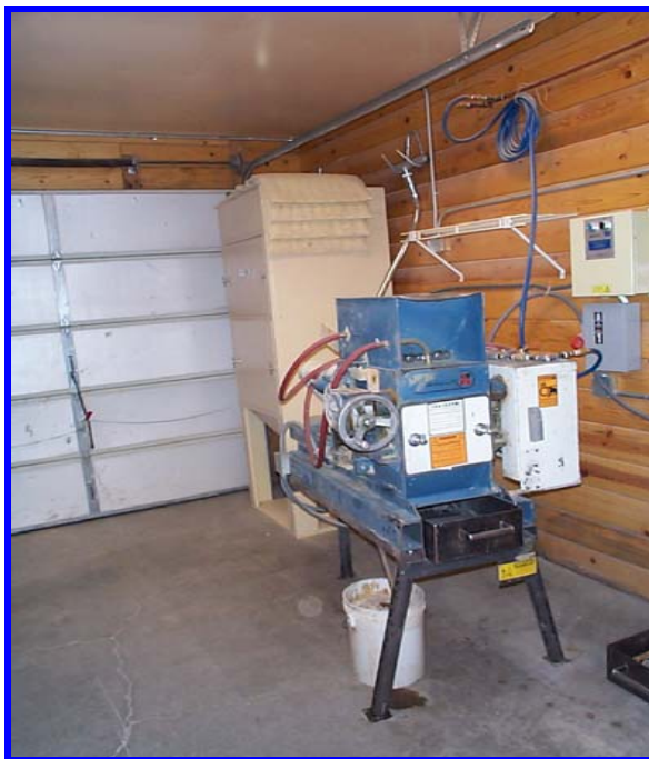
Rosskamp 12 inch roll crusher with dedicated dust collector. Throughput: 30 samples per hour.
